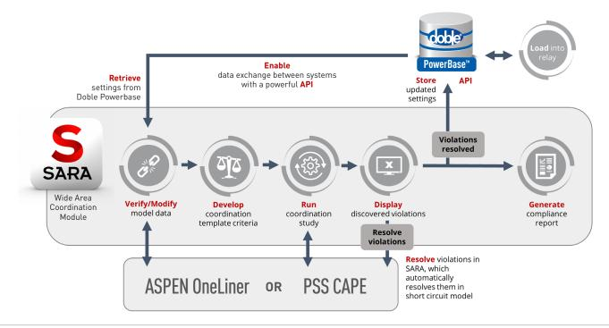
Complying with R2 begins by verifying the model. After SARA retrieves the latest settings from Doble PowerBase, it can then import this data into the short circuit program to verify the model, eliminating the need for manually transporting data between the two programs.
