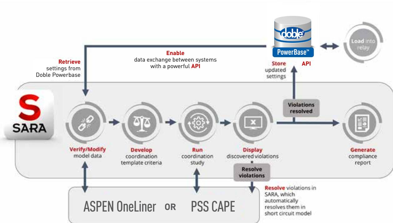
**Complying with R2** begins by verifying the model. After SARA retrieves the latest settings from Doble PowerBase, it can then import this data into the short circuit program to verify the model, eliminating the need for manually transporting data between the two programs.
