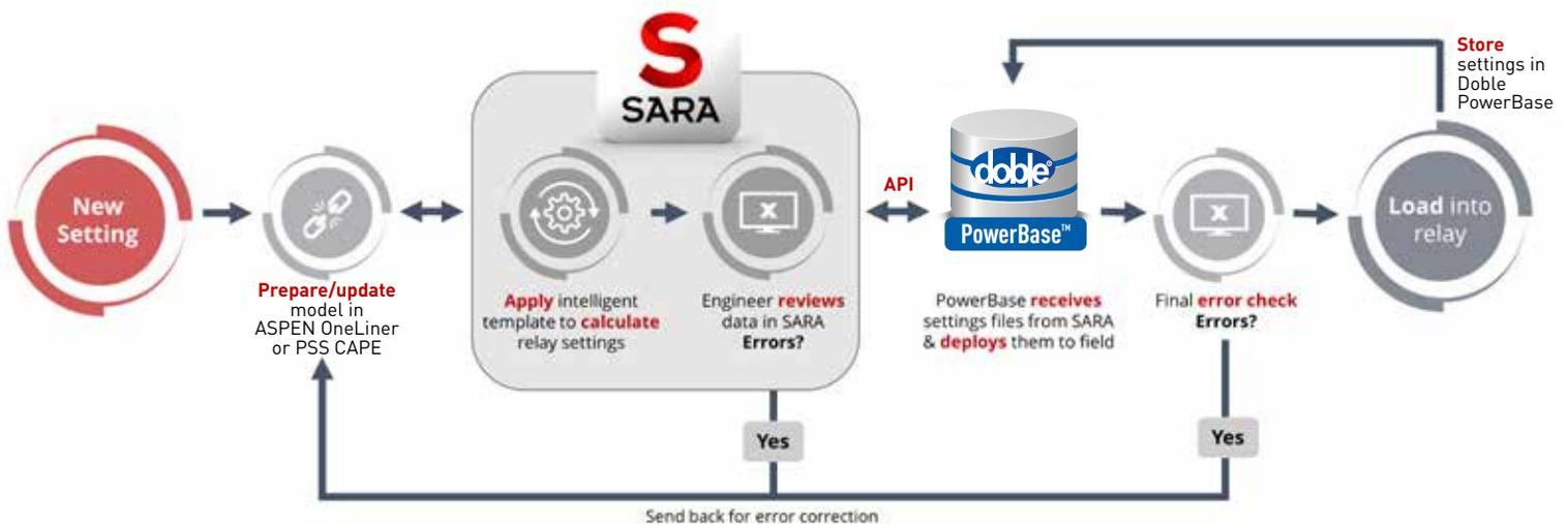
**Complying with R1** begins by preparing the model within a short circuit program such as ASPEN OneLiner or PSS CAPE. The latest data can be automatically retrieved from Doble PowerBase, minimizing time spent preparing new settings.
