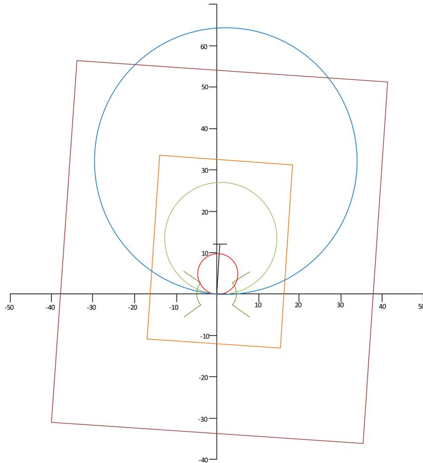
Figure 5. Load Encroachment and OOS Setting for a Long Line
