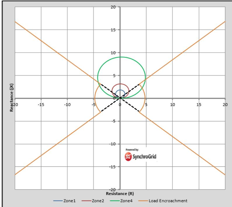
Figure 1. Load Encroachment and mho circle plot
