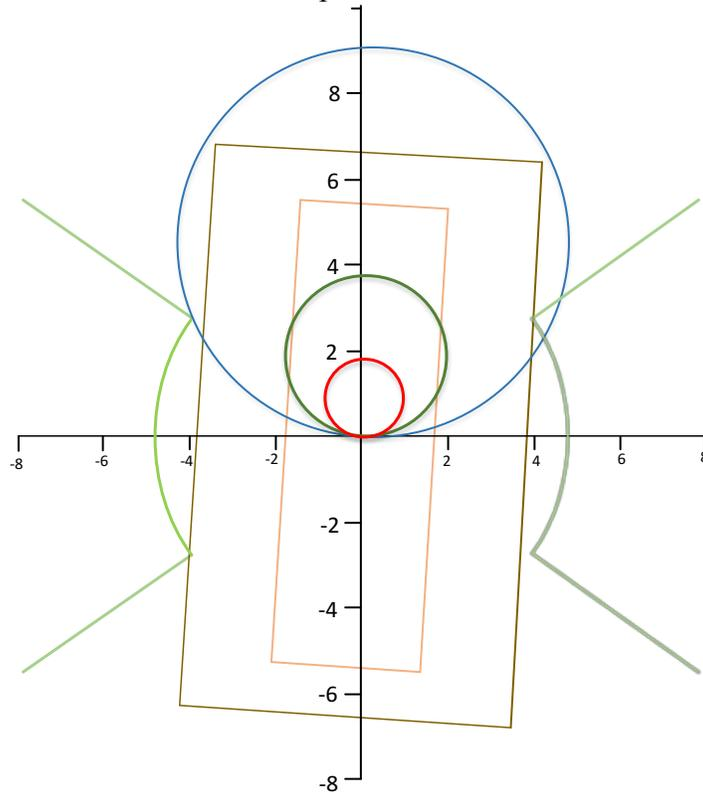
Figure 6. Example of an Incorrect Setting of OOS and Load Encroachment
