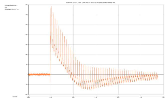
Figure 14. A high magnitude of neutral current flowing during asynchronous reactor switching on 04-10-2018.
