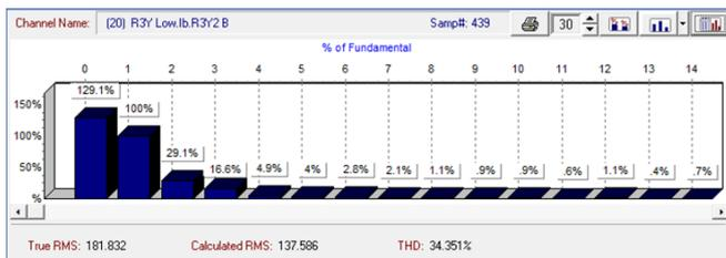
Figure 9. Harmonic analysis of phase B current waveform before CT saturation on 04-10-2018.
