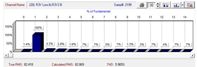
Figure 11. Harmonic analysis of phase B current waveform after CT desaturates on 04-10-2018.
