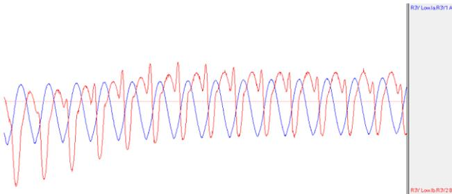
Figure 8. Comparing phase B (saturated) and phase A (unsaturated) current waveforms monitored on 04-10-2018.
