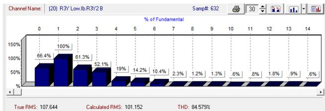
Figure 10. Harmonic analysis of phase B current waveform during CT saturation on 04-10-2018.
