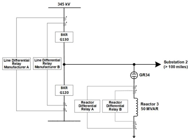
Figure 2. Reactor and line protection arrangement at CTT substation
