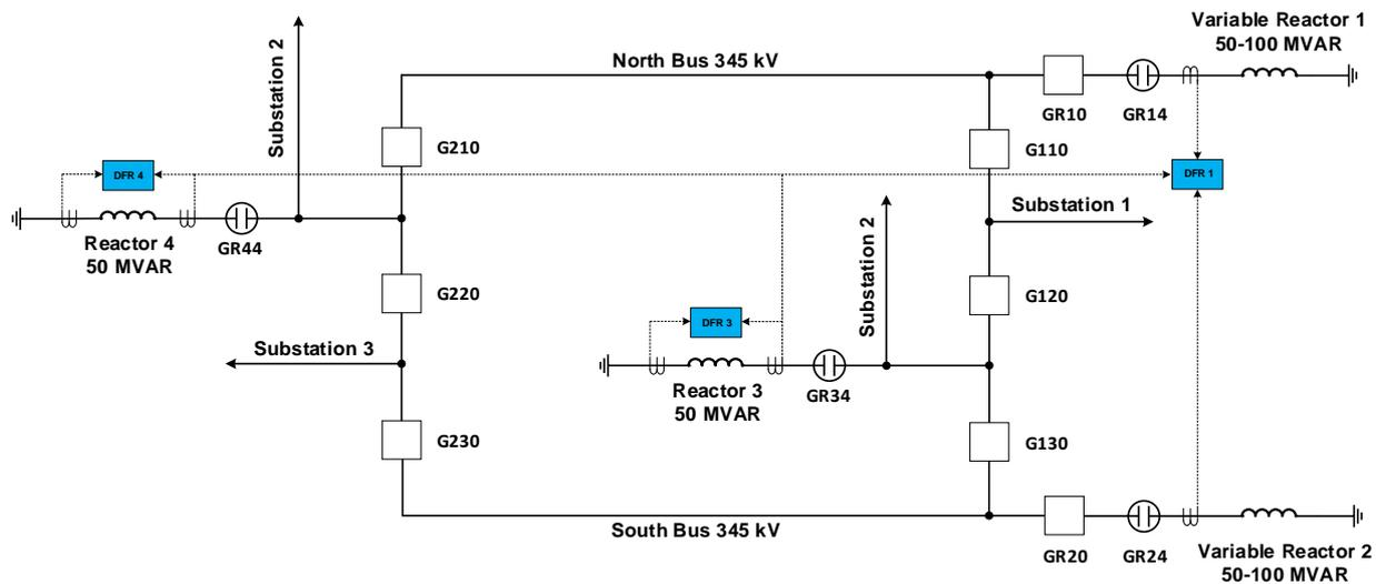
Figure 1. System One-line of CTT substation along with DFR monitoring system in place
