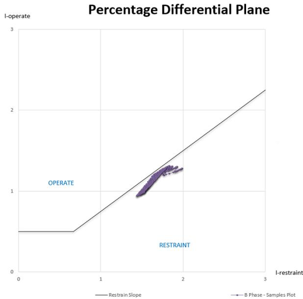
Figure 13. Differential plane showing the instance where CT saturation drives the relay close to the operating region.
