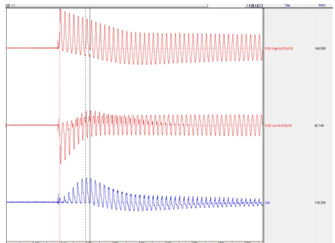
Figure 12. Phase B current waveforms on the high and the low side of shunt reactor where low side CT saturated on 04-10-2018. Resulting calculated differential current is also displayed.
