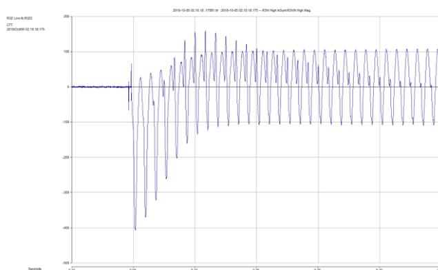
**Figure 7. Phase B current waveform monitored through a saturated CT on 04-10-2018.**
