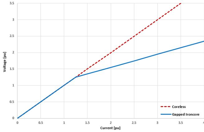
**Figure 3. Magnetization characteristics of Coreless (air-core) and Gapped Iron-core shunt reactors [4]**
