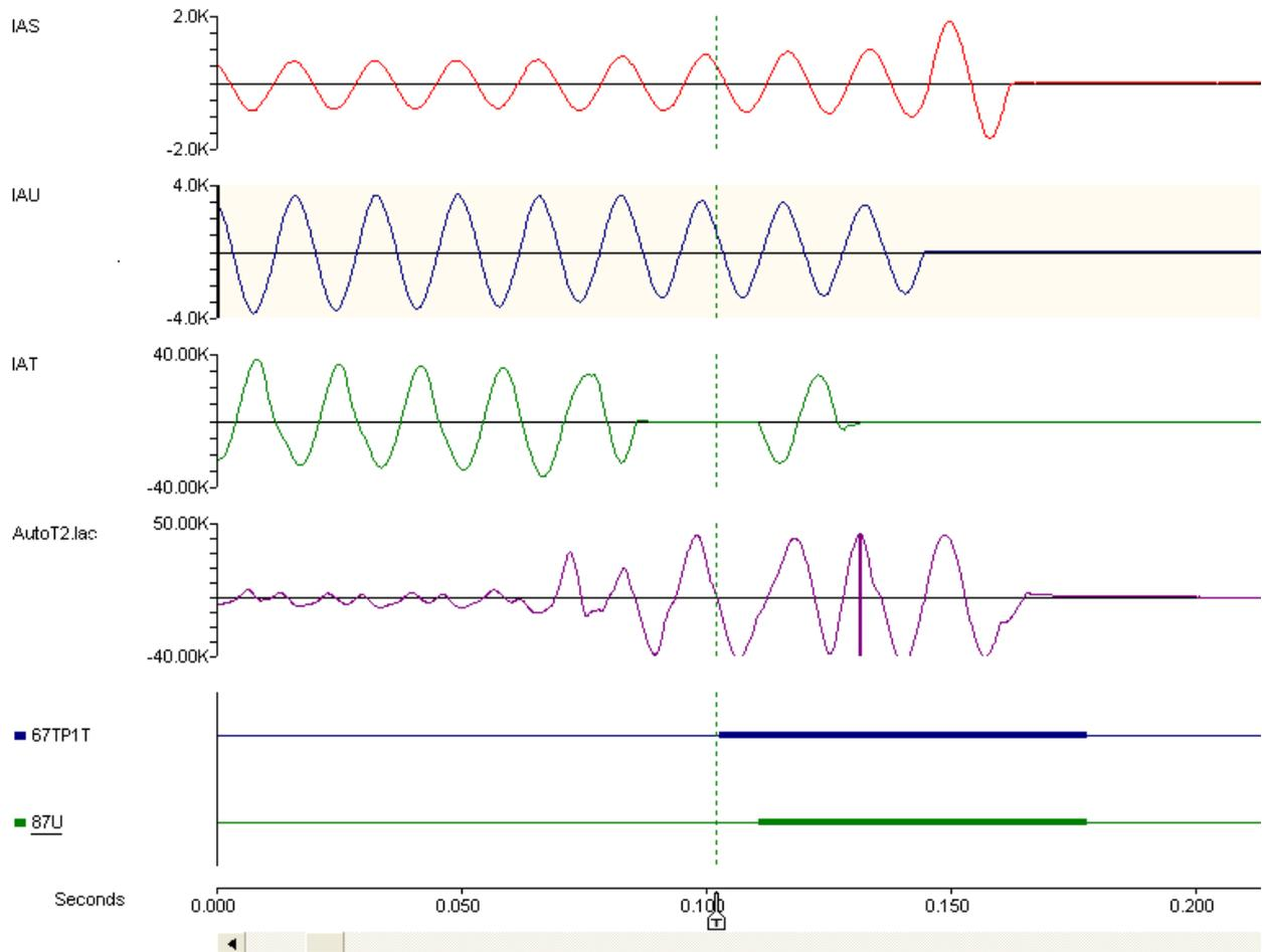
**Figure 3: 87U Differential Operation**
