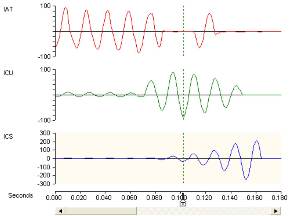
**Figure 8: Fault Energy Transfer from Tertiary IAT to Secondary ICU**
