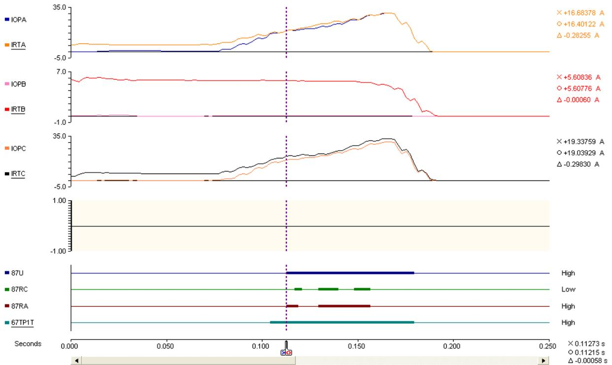
**Figure 4: Operate and Restrain Currents**
