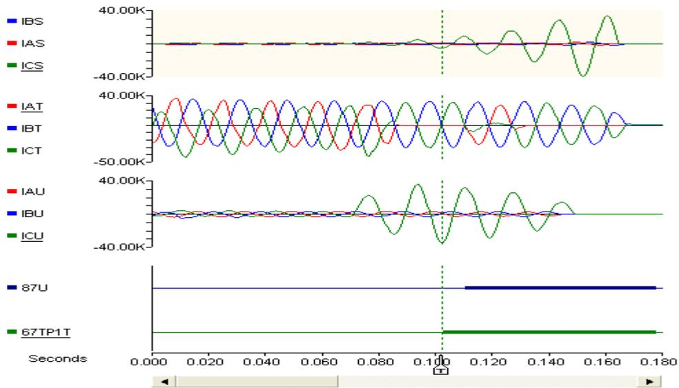
**Figure 7: Differential Relay Operation**
