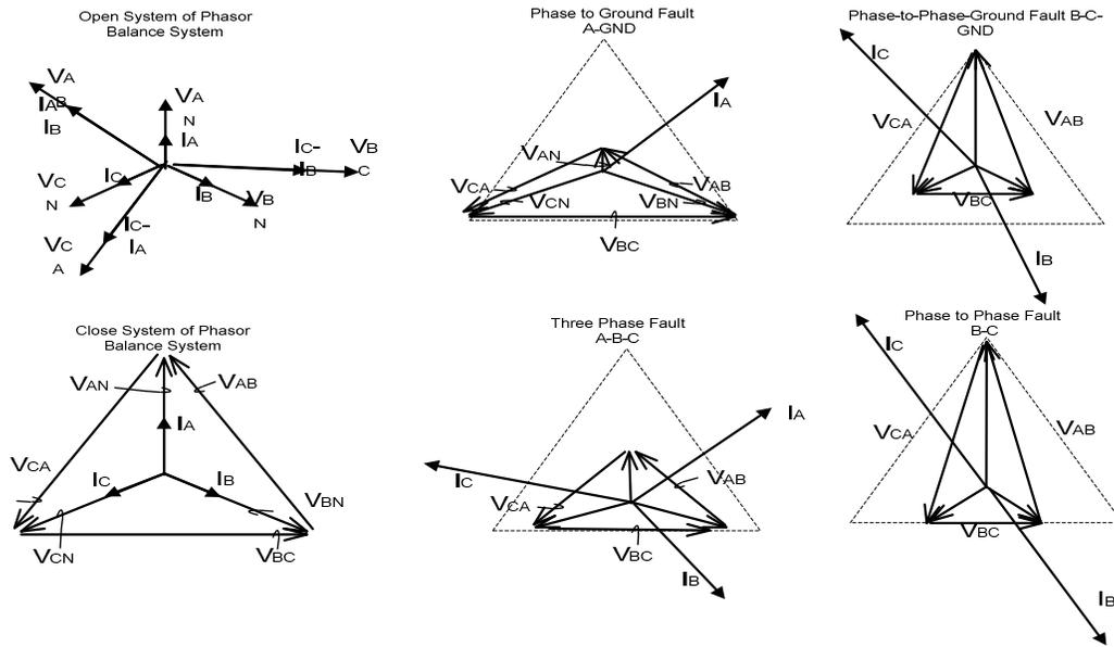
Figure 12. Phasor Representation of Power System Faults.
