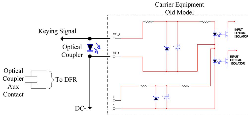
**Figure 11. Use of Optical Coupler with Keying Signal.**
