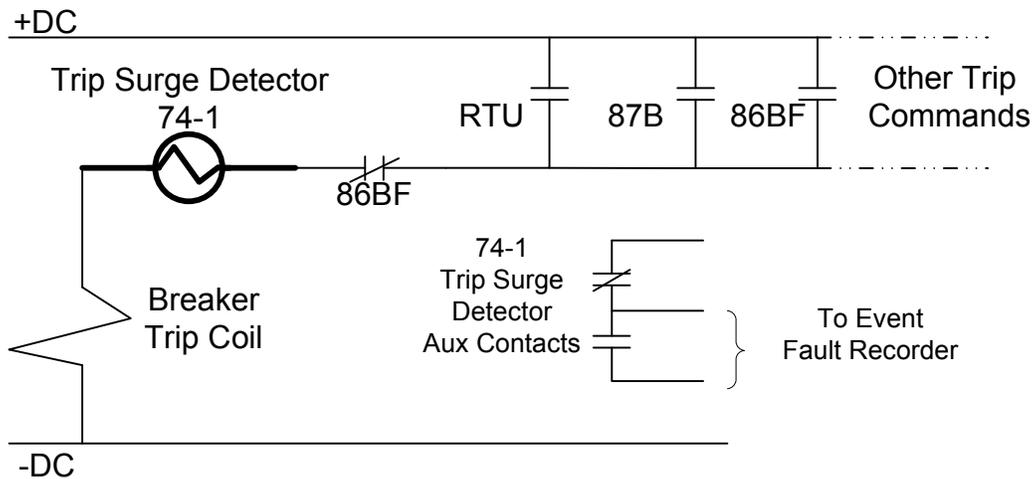
**Figure 9. Trip Surge Detector in Series with Trip Coil.**
