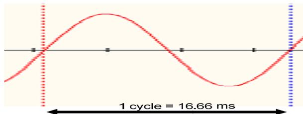
**Figure 4. One Electrical Cycle.**
