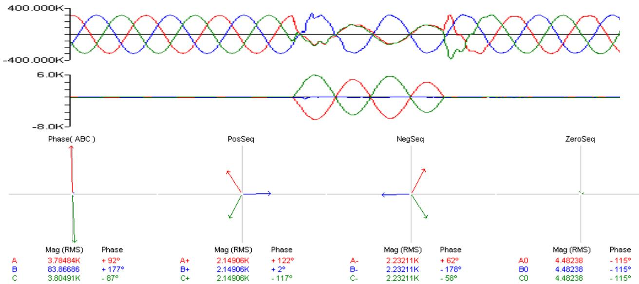
**Figure 14. A-C Phase Fault.**
