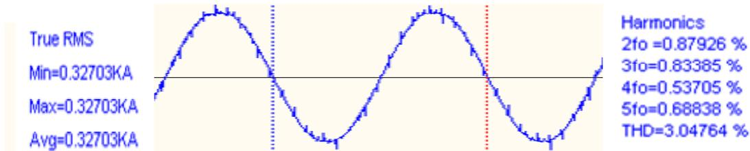
**Figure 5. True RMS Value of Waveform Including Harmonic Content.**
