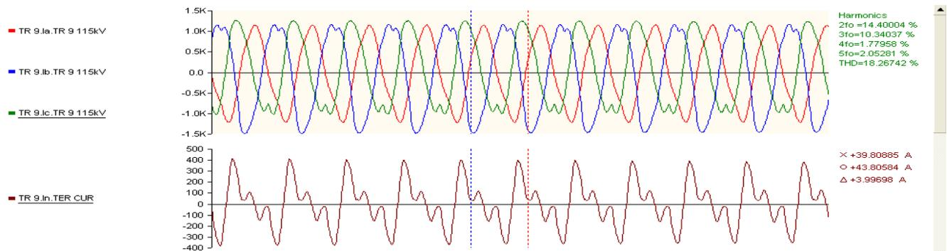
**Figure 7. Currents Behavior during Transformer In-Rush.**
