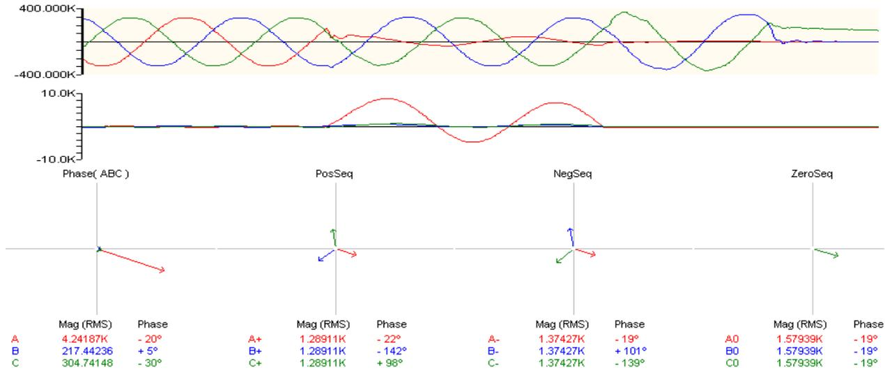
Figure 13. Phase A to Ground Fault.
