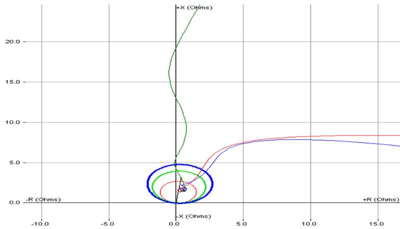
**Figure 17. Fault Impedance Trajectory Superimposed With Zone Mho Circles.**
