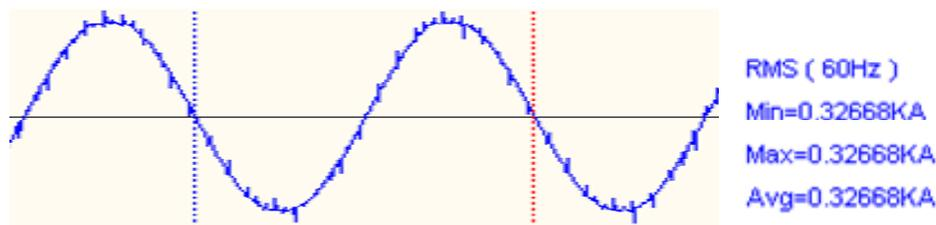
**Figure 6. Fundamental RMS Value of Waveform with No Harmonic Content.**
