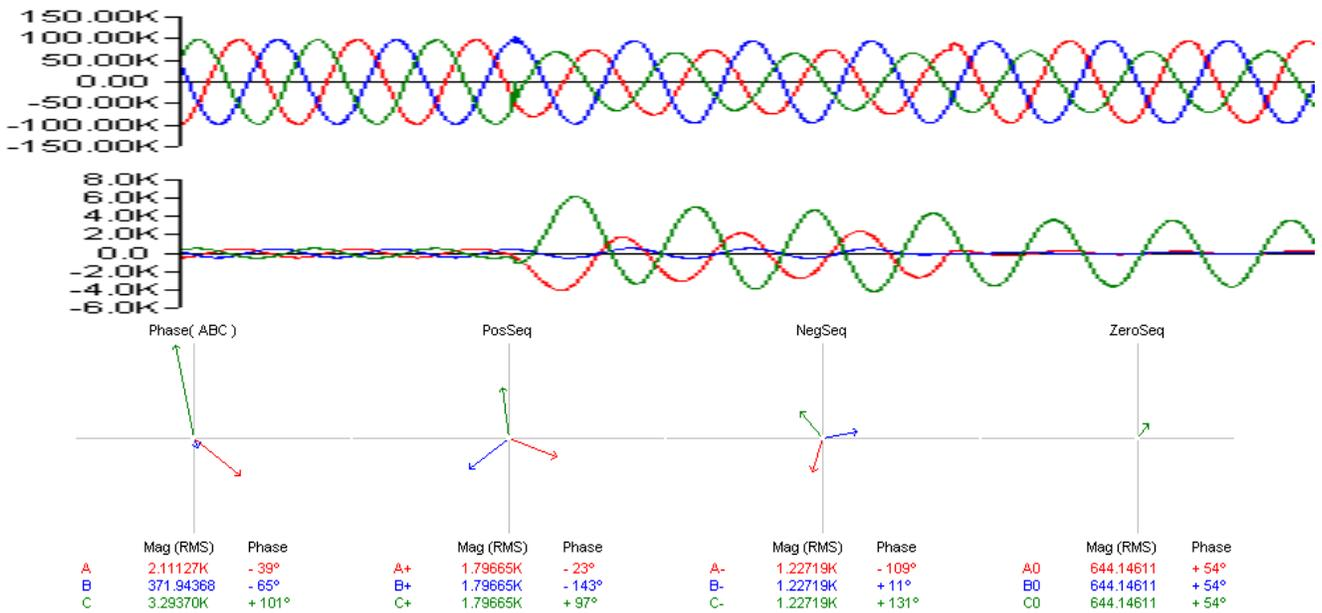
**Figure 15. A-C-Ground Fault.**
